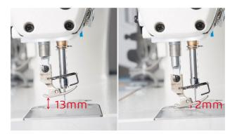
After trimming and midway, the height of the presser foot can be adjusted within the range of 0-13mm, which can meet the requirements of different fabrics, saving labor and convenience.
